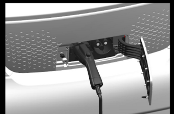
Efficient fast charge + home slow charge: Dual charging ports with dual temperature control protection.
